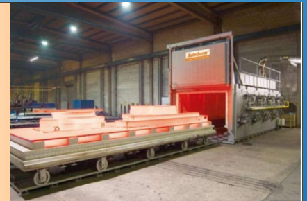
Bogie Hearth Furnaces / Movable Bogie Furnaces Car Bottom Furnace / Pull Out Furnaces
